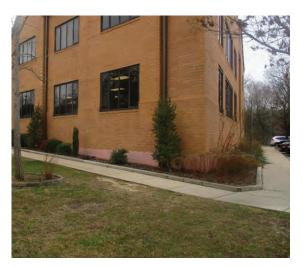
Parking spaces in the parking lot to the south of the building can be converted to porous pavement to capture and infiltrate stormwater runoff from the parking lot. Additional space west of the building can be converted to capture stormwater from the rooftop. This water can first be partially treated with a series of stormwater planters. A preliminary soil assessment suggests that the soils have suitable drainage characteristics for green infrastructure.
