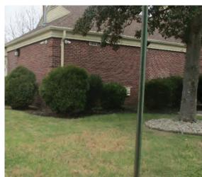
Two rain gardens can be installed at the southeast end of the building by redirecting downspouts into them to capture, treat, and infiltrate stormwater runoff from the rooftop. A preliminary soil assessment suggests that the soils have suitable drainage characteristics for green infrastructure.
