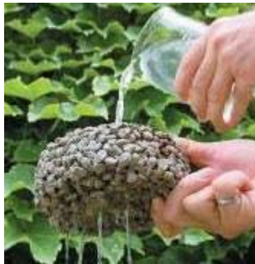
Figure 19: Example of pervious concrete allowing water to flow through it 1
