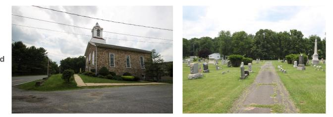
Rainwater from the church parking lot drains onto the road. A rain garden could be built south of the lot to capture, treat, and infiltrate runoff. Additionally, the cracked paved walkway in the cemetery could be replaced with porous asphalt to allow water to infiltrate. A preliminary soil assessment suggests that the soils have suitable drainage characteristics for green infrastructure.
