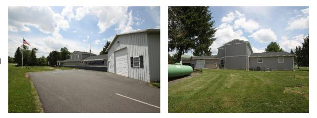
There is an existing detention basin. South of the building there is an opportunity for a rain garden to be built to capture, treat, and infiltrate stormwater. A cistern can be installed north of the building to harvest rainwater to be used to wash vehicles. A preliminary soil assessment suggests that the soils have suitable drainage characteristics for green infrastructure.
