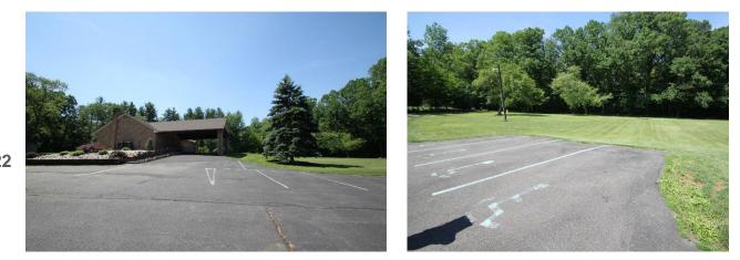
Rainwater drains into the lawn area west of the building. A rain garden can be built on the lawn to capture, treat, and infiltrate roof and parking lot runoff. The parking spaces southwest of the building can be replaced with porous asphalt to allow stormwater to infiltrate. A preliminary soil assessment suggests that the soils have suitable drainage characteristics for green infrastructure.
