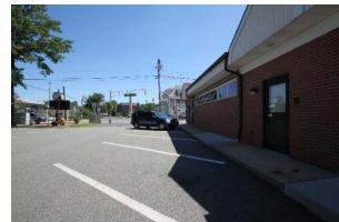
Runoff from the site currently flows onto a parking lot beside the building. Several downspouts can be connected to a cistern to harvest this water. Parking spots can also be replaced with porous asphalt to capture and infiltrate runoff as well. A preliminary soil assessment suggests that soils have suitable drainage characteristics for green infrastructure.
