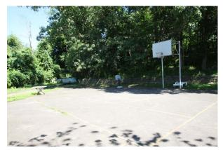
Several disconnected downspouts direct water onto existing porous pavement. A lot of runoff also flows onto the basketball court at the corner of the site, which could be replaced with porous pavement. A preliminary soil assessment suggests that more soil testing would be required before determining soil suitability for green infrastructure.
