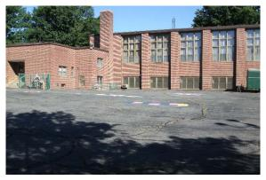
Water on the site currently pools in the parking lot behind the building complex. The lot behind the school can be partially de-paved into a lawn area to address the pooling. Pedestrian walkways can be replaced with porous pavement to capture runoff. A rain garden can also be planted at the back of the site to capture roof runoff and serve as an educational opportunity for students. A preliminary soil assessment suggests that soils have suitable drainage characteristics for green infrastructure.
