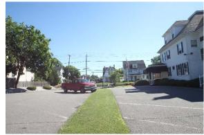
Water currently drains from the parking lot towards the building. The grass buffer in the parking lot can be converted to a rain garden to capture and treat runoff. The sidewalk can be replaced with porous pavement to infiltrate runoff as well. A preliminary soil assessment suggests that soils have suitable drainage characteristics for green infrastructure.
