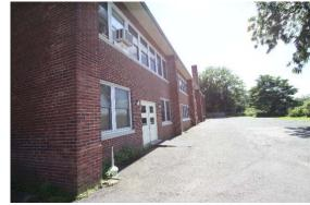
Runoff from the roof of the preschool currently drains onto pavement behind the building. The lawn area at the front can be converted into two rain gardens to capture and infiltrate this roof runoff. Downspouts may be redirected into rain barrels as well to harvest rainwater that could be used to water existing gardens behind the school. A preliminary soil assessment suggests that soils have suitable drainage characteristics for green infrastructure.
