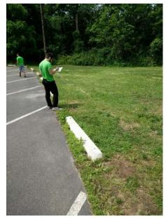
Water from the entire site currently drains into a body of water behind the building. The grass area between the water and the parking lot can be converted into a rain garden to capture and treat this runoff. A preliminary soil assessment suggests that more soil testing would be required before determining soil suitability for green infrastructure.
