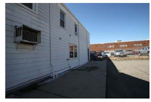
Runoff from the parking lot is currently directed towards an adjacent southeast building. Parking spots can be replaced with porous asphalt to capture and infiltrate this runoff. A preliminary soil assessment suggests that soils have suitable drainage characteristics for green infrastructure.
