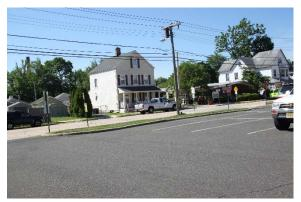
Runoff from the parking lot currently drains toward the street. The grass buffer in the parking lot can be replaced with a rain garden to capture, infiltrate, and treat this runoff. Additionally, areas behind the school can be de-paved into lawn and the basketball courts can be replaced with porous pavement. A preliminary soil assessment suggests that soils have suitable drainage characteristics for green infrastructure.
