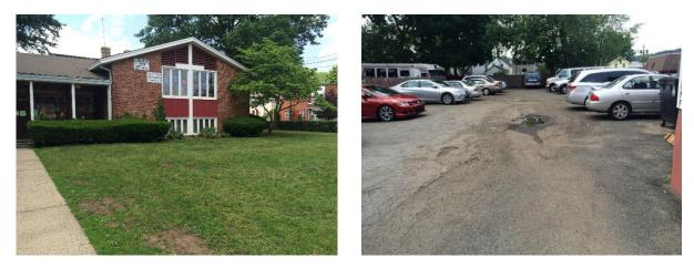
Parking spaces can be replaced with pervious pavement to capture and infiltrate stormwater. Two rain gardens can also be built in front of the church to capture, treat, and infiltrate runoff from the roof. A preliminary soil assessment suggests that more soil testing would be required before determining the soil's suitability for green infrastructure.
