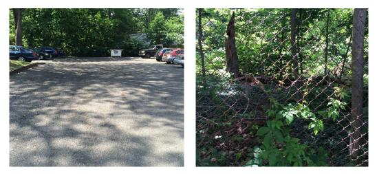
Parking spaces can be converted into pervious pavement to capture and infiltrate runoff before it flows into the stream behind the library. Stormwater planters can also be installed in front of the library to intercept stormwater from the roadway. A preliminary soil assessment suggests that the soils have suitable drainage characteristics for green infrastructure.
