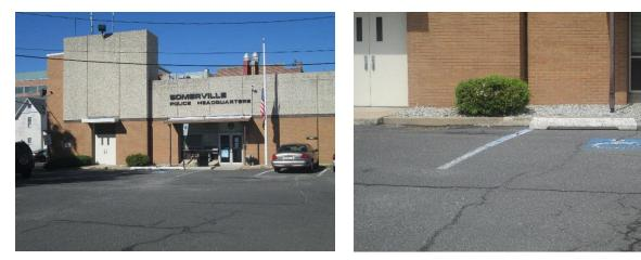
Parking spaces can be converted into pervious pavement to infiltrate stormwater runoff from the surrounding paved surfaces as well as the downspouts that are currently draining onto the lot. A preliminary soil assessment suggests that the soils have suitable drainage characteristics for green infrastructure.
