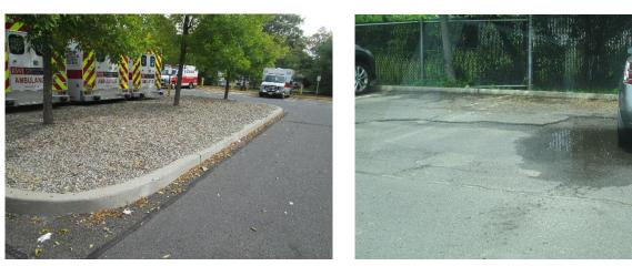
Parking spaces can be replaced with pervious pavement to capture and infiltrate stormwater. A preliminary soil assessment suggests that more soil testing would be required before determining soil suitability for green infrastructure.
