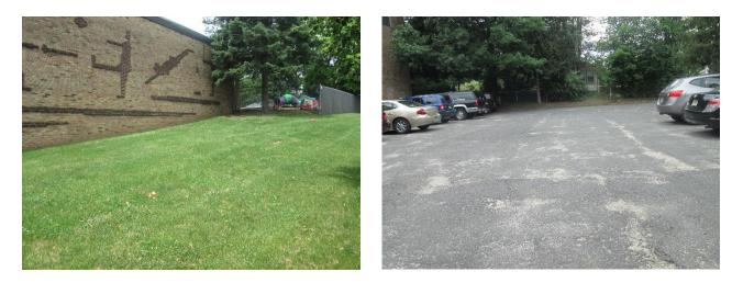
Parking spaces can be replaced with pervious pavement to infiltrate stormwater and reduce impervious cover. A preliminary soil assessment suggests that the soils have suitable drainage characteristics for green infrastructure.
