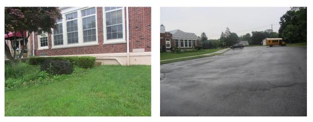
Parking spots can be replaced with porous asphalt to capture and infiltrate stormwater generated by the parking lots. Bioretention systems can be installed to capture, treat, and infiltrate rooftop runoff from the northeast side of the school and playground runoff from the northwest side of the site. Two downspouts can be disconnected and redirected into a rain garden. A preliminary soil assessment suggests that the soils have suitable drainage characteristics for green infrastructure.
