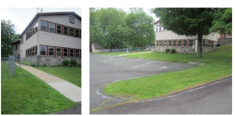
Parking spots at the church can be replaced with porous asphalt to capture and infiltrate stormwater. A preliminary soil assessment suggests that the soils have suitable drainage characteristics for green infrastructure.
