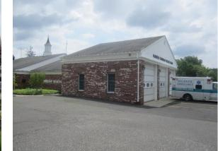
Parking spots around the complex can be replaced with porous asphalt to capture and infiltrate stormwater. A preliminary soil assessment suggests that the soils have suitable drainage characteristics for green infrastructure.
