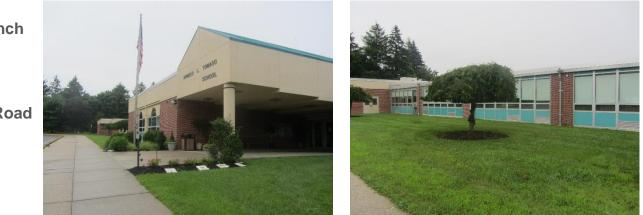
Rows of parking spots around the school can be replaced with porous asphalt to capture and infiltrate stormwater. In the turf grass on the northeast side of the school a rain garden can be installed to capture, treat, and infiltrate roof runoff. A preliminary soil assessment suggests that more soil testing would be required before determining the soil's suitability for green infrastructure.
