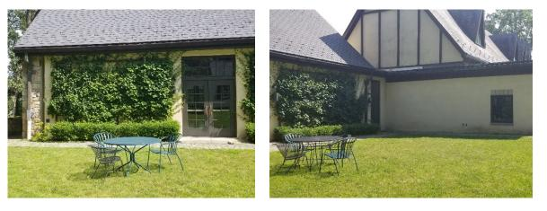
Rain gardens can be installed at the corner of the sidewalk and adjacent to the shed to the north of the church to capture, treat, and infiltrate rooftop runoff. Downspout planter boxes can be installed at the northeast corner of the building to capture and filter stormwater. A preliminary soil assessment suggests that more soil testing would be required before determining the soil's suitability for green infrastructure.
