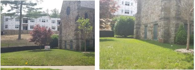
A rain garden can be installed along the southeast side of the church and at the bottom of a hill on the property to capture, treat, and infiltrate parking lot and rooftop runoff. A preliminary soil assessment suggests that more soil testing would be required before determining the soil's suitability for green infrastructure.
