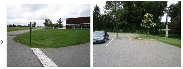
Parking spaces in the parking lot to the northeast of the building can be converted to porous pavement to capture and infiltrate stormwater runoff from the parking lot. A rain garden can be installed near the catch basin and entrance of the building to capture, treat, and infiltrate stormwater runoff from the roof. A preliminary soil assessment suggests that the soils have suitable drainage characteristics for green infrastructure.
