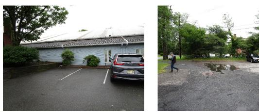
Parking spaces in the parking lot to the south of the building can be converted to porous pavement to capture and infiltrate stormwater runoff from the roof via the downspouts, which are disconnected. A preliminary soil assessment suggests that more soil testing would be required before determining the soil's suitability for green infrastructure.
