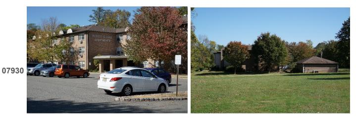
Two rain gardens can be installed west of the two buildings to accumulate and infiltrate stormwater runoff from the buildings. Additionally, porous pavement can be used to capture stormwater from the parking lot in front of the main building. A preliminary soil assessment suggests that more soil testing would be required before determining the soil's suitability for green infrastructure.
