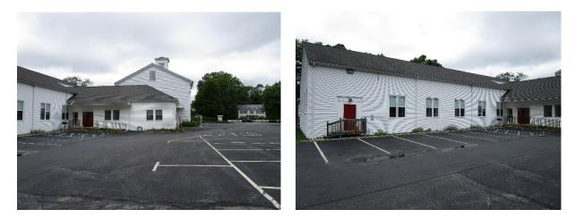
Parking spaces in the parking lot to the southwest of the building can be converted to porous pavement to capture and infiltrate stormwater runoff from the parking lot and downspouts. A preliminary soil assessment suggests that the soils have suitable drainage characteristics for green infrastructure.
