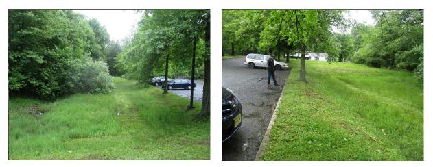
A rain garden can be installed to reduce the flooding that occurs east of the parking lot. Pervious pavement can be installed in the parking lot row directly west of the building to capture stormwater runoff from both the parking lot and the rooftop. A preliminary soil assessment suggests that more soil testing would be required before determining the soil's suitability for green infrastructure.
