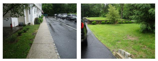
A rain garden can be installed south of the roadway to capture, treat, and infiltrate stormwater runoff from the pavement. Downspout planter boxes can be installed along the front, southern wall of the building to capture stormwater runoff from the rooftop. A preliminary soil assessment suggests that the soils have suitable drainage characteristics for green infrastructure.
