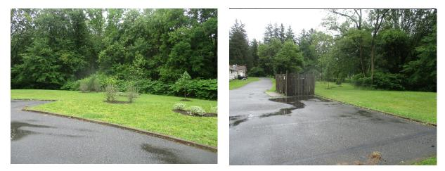
Pervious pavement can be installed in the western corner of the parking lot to capture and infiltrate stormwater runoff from the parking lot. A rain garden can be installed along the roadway south of the building to capture stormwater runoff from the pavement. A preliminary soil assessment suggests that more soil testing would be required before determining the soil's suitability for green infrastructure.
