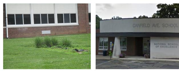
A rain garden can be installed near the disconnected downspouts to capture, treat, and infiltrate rooftop runoff. A preliminary soil assessment suggests that more soil testing would be required before determining the soil's suitability for green infrastructure.
