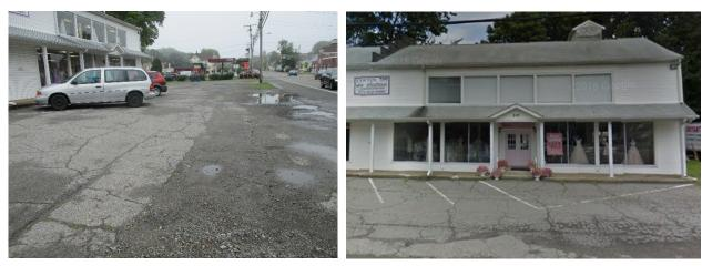
Pervious pavement can be installed on a parking strip south of the building to capture and infiltrate stormwater. A preliminary soil assessment suggests that the soils have suitable drainage characteristics for green infrastructure.
