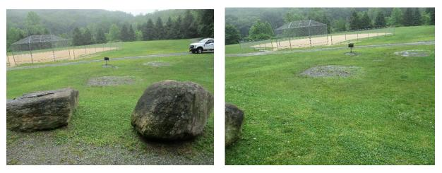
A rain garden can be installed in the turfgrass area on the north side of the park to capture, treat, and infiltrate stormwater runoff from the parking/roadway area. A preliminary soil assessment suggests that more soil testing would be required before determining the soil's suitability for green infrastructure.
