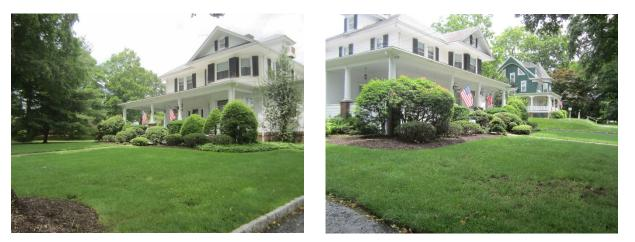
Rain gardens can be installed in front of the building, on either side of the walkway to help capture, treat, and infiltrate rooftop runoff. Pervious pavement can be installed on the northwest side of the home to infiltrate and filter parking lot runoff. A preliminary soil assessment suggests that more soil testing would be required before determining the soil's suitability for green infrastructure.
