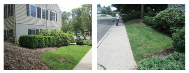
A rain garden can be installed adjacent to the sidewalk and north of the building to capture, treat, and infiltrate stormwater runoff from the roof of the building. Pervious pavement can be installed in the southeastern corner of the parking lot to infiltrate pavement runoff. A preliminary soil assessment suggests that more soil testing would be required before determining the soil's suitability for green infrastructure.
