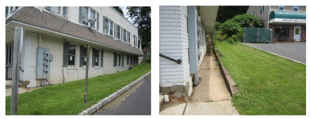
A rain garden can be installed between the post office and the parking lot to capture, treat, and infiltrate rooftop runoff since no gutters are installed. A preliminary soil assessment suggests that more soil testing would be required before determining the soil's suitability for green infrastructure.
