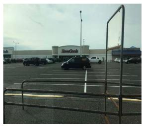
Sections of parking spaces can be converted to porous pavement to capture and infiltrate stormwater runoff from the parking lot. A parking lot island can be converted to a rain garden to capture, treat, and infiltrate stormwater runoff from the parking lot as well. A preliminary soil assessment suggests that the soils have suitable drainage characteristics for green infrastructure.
