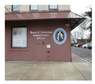
A section of sidewalk can be converted to a stormwater planter to capture, treat, and infiltrate stormwater runoff from the Board of Education's building roof and sidewalk. A preliminary soil assessment suggests that more soil testing would be required before determining the soil's suitability for green infrastructure.
