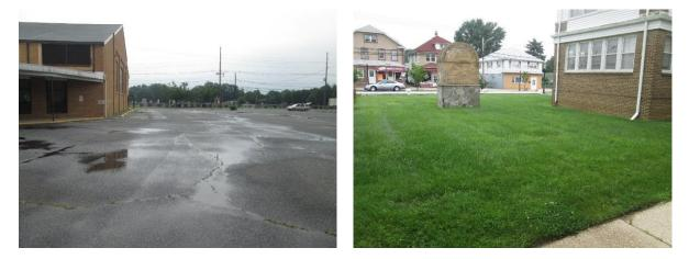
Parking spots can be replaced with porous asphalt to capture and infiltrate stormwater. A rain garden can be installed adjacent to the building to capture, treat, and infiltrate roof runoff. A preliminary soil assessment suggests that the soils have suitable drainage characteristics for green infrastructure.
