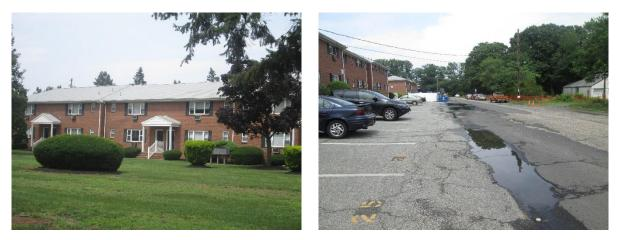
Parking spots can be replaced with porous asphalt to capture and infiltrate stormwater. Multiple rain gardens can be installed throughout the complex adjacent to the buildings to capture, treat, and infiltrate roof runoff. A preliminary soil assessment suggests that the soils have suitable drainage characteristics for green infrastructure.
