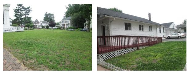
Parking spaces can be replaced with porous asphalt to capture and infiltrate stormwater. Installing rain gardens adjacent to the building can capture, treat, and infiltrate roof runoff. A preliminary soil assessment suggests that more soil testing would be required before determining the soil's suitability for green infrastructure.
