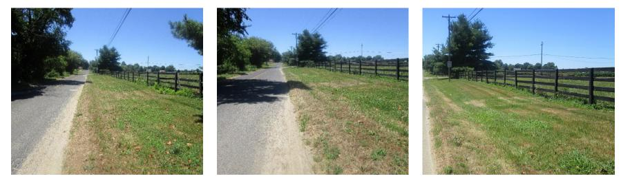
Bioswales can be installed along the fence pictured above to capture stormwater runoff from the road. The turfgrass areas alongside the road are eroding due to the flow of the runoff. These areas are also at a lower depth than that of the road, which would allow the stormwater to flow into the bioswales. A preliminary soil assessment suggests that the soils have suitable drainage characteristics for green infrastructure.
