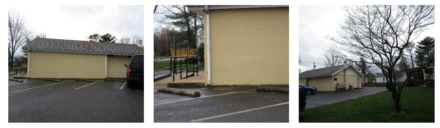
The parking spaces along the south side of the building can be converted into pervious pavement to allow stormwater runoff from the roof and pavement to infiltrate the ground. Downspout planter boxes can be installed on the north side of the building to capture runoff from the roof and enhance the aesthetic of the building. A preliminary soil assessment suggests that more soil testing would be required before determining the soil's suitability for green infrastructure.
