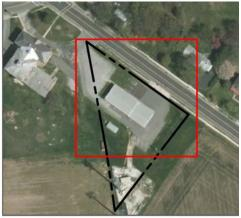
bioretention system rainwater harvesting [] drainage area [] property line 2015 Aerial: NJOIT, OGIS
