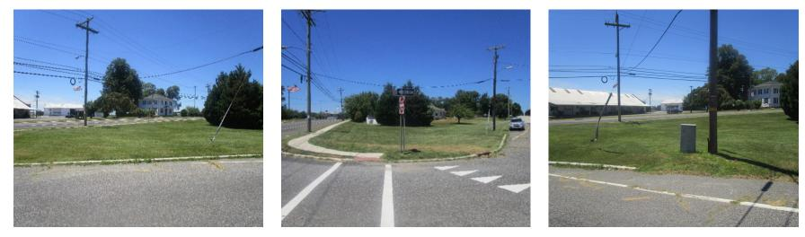
The turfgrass area is at a lower elevation than the road; curb cuts can be made to allow stormwater to flow into a rain garden. This system will manage stormwater runoff from the road, enhance the aesthetic of the area, and create a habitat for wildlife. A preliminary soil assessment suggests that the soils have suitable drainage characteristics for green infrastructure.
