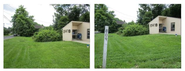
A rain garden can be installed at the front of the property to collect stormwater runoff from the building as well as from the road near the property. A preliminary soil assessment suggests that the soils have suitable drainage characteristics for green infrastructure.
