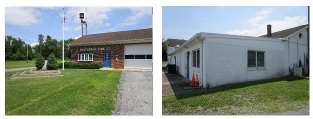
A rain garden can be installed along the north side of the building to manage rooftop runoff. A rainwater harvesting system can be installed at the northwest corner of the building to capture stormwater runoff from the roof as well. This can be used to clean fire trucks and for other non-potable purposes. A preliminary soil assessment suggests that more soil testing would be required before determining the soil's suitability for green infrastructure.
