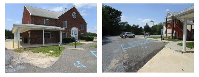
A rain garden can be installed at the front of the building to capture, treat, and infiltrate rooftop runoff. Two sections of parking spaces can be converted to porous pavement to capture and infiltrate stormwater runoff from the roof and the parking lot. A preliminary soil assessment suggests that more soil testing would be required before determining the soil's suitability for green infrastructure.
