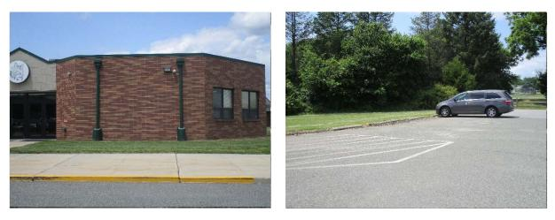
Two rain gardens can be installed at the east and west ends of the building to capture, treat, and infiltrate stormwater runoff from the roof. A section of parking spaces can be converted to porous pavement to collect and infiltrate stormwater from the parking lot. A preliminary soil assessment suggests that more soil testing would be required before determining the soil's suitability for green infrastructure.
