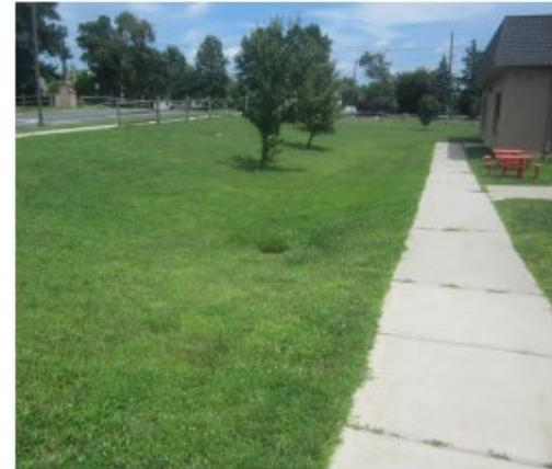
Stormwater is currently directed to existing catch basins. Parking spots by the north and west buildings can be replaced with porous asphalt to capture and infiltrate stormwater runoff from the parking lot. Rain gardens adjacent to the building can capture, treat, and infiltrate roof runoff before it reaches the existing catch basin. A preliminary soil assessment suggests that the soils have suitable drainage characteristics for green infrastructure.
