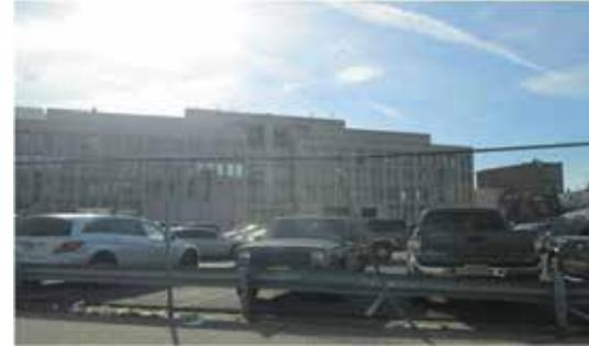
The site is the Paterson Municipal Court located at 111 Broadway. The site slopes from the north to south. The building has no external downspouts. There is an area of grass with a storm drain in it; a bioswale or rain garden can be implemented to capture sidewalk runoff before it reaches the drain. The rear parking lot of the building was inaccessible.
