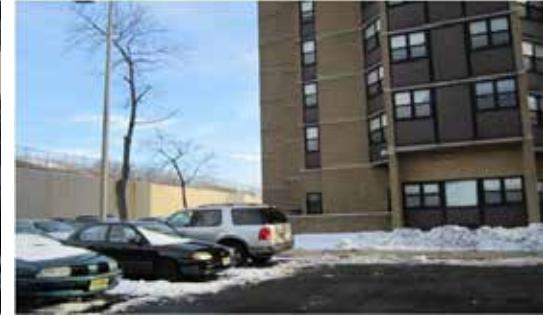
The site is the Governor Residential Apartments located at 27 State Street. The site has a slope from the southwest to northeast. There is also a slight slope north. There are islands in the parking lot that can be converted into bioswales. The sidewalk slopes directly into the parking lot; a rain garden can be placed next to it to divert rainwater from the impervious surface. There is also a courtyard in the center of the complex in which a rain garden or a bioswale can be installed.
