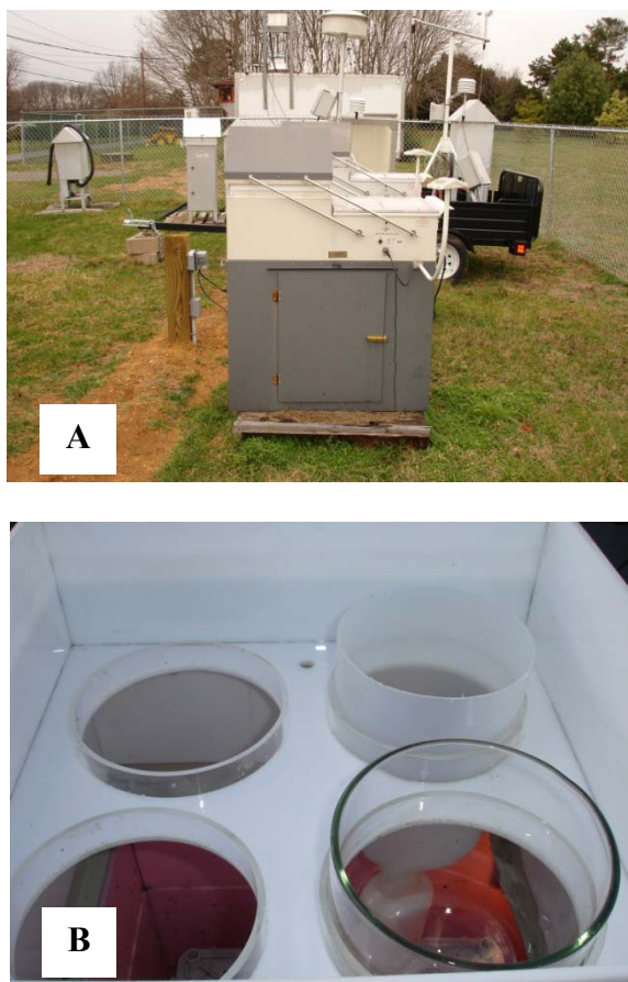
Figure 2.2 A) MIC-B wet deposition collector in fenced area at Rutgers Gardens, NJ. B) Wet deposition assemblies with acrylic support inserts [Landis & Keeler 1997] inside the MIC-B wet deposition collector. Trace element funnel located far right and total mercury funnel located near right.
