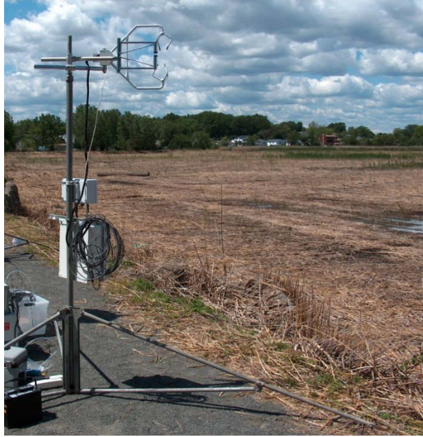
Figure 3.2 Eddy correlation system at the Secaucus High School Marsh 10-11 August 2005 ( Phragmites removed).
