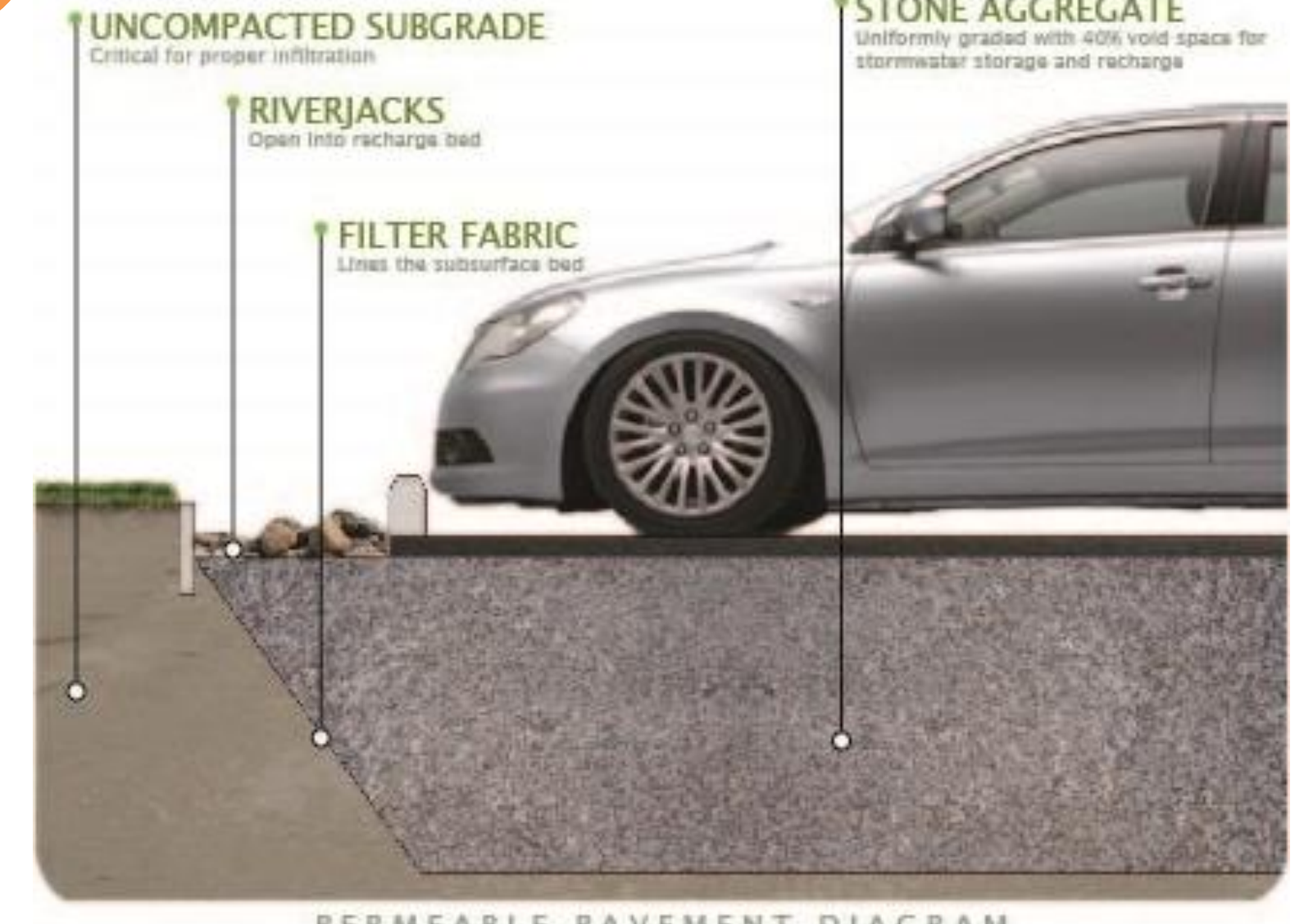
PERMEABLE PAVEMENT DIAGRAM
