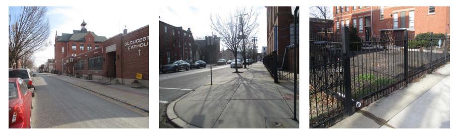
Stormwater is currently draining from north to south across the site. Stormwater planters can be installed along the northern and southern sidewalks to capture and treat stormwater runoff. A preliminary soil assessment suggests that more soil testing would be required before determining the soil's suitability for green infrastructure.
