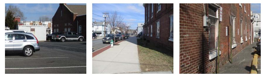
Stormwater is currently draining from south to north across the site. Parking spaces in the east lot can be converted to porous asphalt to capture and treat stormwater runoff. Adjacent downspouts along the building can also be directed into the parking lot, allowing for the treatment of roof runoff. A preliminary soil assessment suggests that more soil testing would be required before determining the soil's suitability for green infrastructure.
