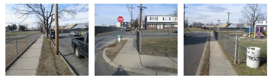
Stormwater is currently draining from south to north across the site. Tree filter boxes can be constructed along the northern sidewalk to capture and treat stormwater runoff and provide additional landscape value to the site. Adjacent sidewalks can be converted to porous asphalt to capture and treat stormwater runoff. A preliminary soil assessment suggests that more soil testing would be required before determining the soil's suitability for green infrastructure.
