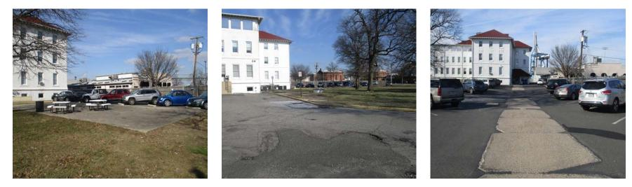
Stormwater is currently draining across the site into nearby catch basins. Parking spaces in the east lot can be converted to porous asphalt to capture and treat stormwater runoff. Stormwater can be diverted from the main parking lot into a rain garden. Installing a rain garden adjacent to the parking lot can capture, treat, and infiltrate runoff. A preliminary soil assessment suggests that more soil testing would be required before determining the soil's suitability for green infrastructure.
