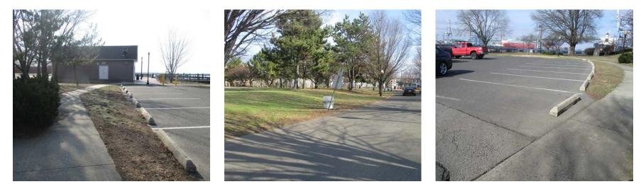
Stormwater is currently draining from east to west across the site. Parking spaces in the Proprietors Park parking lot can be converted to porous asphalt to capture and treat stormwater runoff. Stormwater can be diverted from the road into a rain garden. Installing a rain garden adjacent to the roadway can capture, treat, and infiltrate runoff. A preliminary soil assessment suggests that more soil testing would be required before determining the soil's suitability for green infrastructure.
