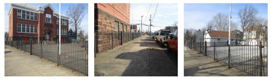
Stormwater is currently draining across the site to nearby catch basins. Tree filter boxes can be constructed along the southern sidewalk to capture and treat stormwater runoff and provide additional landscape value to the site. The paved area adjacent to the main entrance can be converted to porous asphalt to capture and treat stormwater runoff. A preliminary soil assessment suggests that more soil testing would be required before determining the soil's suitability for green infrastructure.
