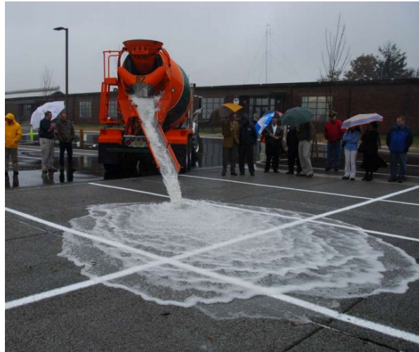
Figure 2: Rapid infiltration of water through porous pavement is demonstrated at the USEPA Edison New Jersey test site
