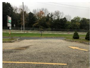
Parking spaces in the parking lot to the east of the building can be converted to porous pavement to capture and infiltrate stormwater runoff from the parking lot. A bioretention system can be installed in the island south of the building to capture, treat, and infiltrate stormwater runoff from the parking lot. A preliminary soil assessment suggests that more soil testing would be required before determining the soil's suitability for green infrastructure.
