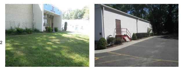
Parking spots south of the building can be replaced with porous asphalt to capture and infiltrate stormwater. Downspouts along the building can be disconnected and directed into porous asphalt parking spaces in order to decrease runoff. A preliminary soil assessment suggests that more soil testing would be required before determining the soil's suitability for green infrastructure.
