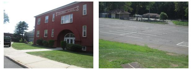
Parking spots south of the school can be replaced with porous asphalt to capture and infiltrate stormwater. A preliminary soil assessment suggests that more soil testing would be required before determining the soil's suitability for green infrastructure.
