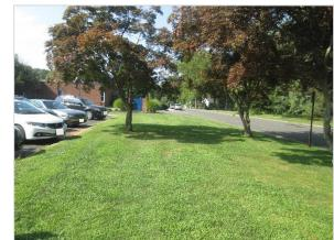
Parking spots to the east and west of the building can be replaced with porous asphalt to capture and infiltrate stormwater. Installing a rain garden adjacent to the building can capture, treat, and infiltrate roof runoff. A preliminary soil assessment suggests that the soils have suitable drainage characteristics for green infrastructure.
