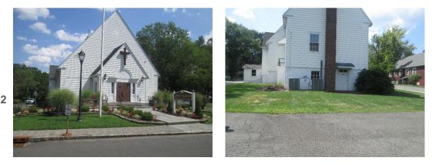
Parking spots east of the building can be replaced with porous asphalt to capture and infiltrate stormwater. A rain garden can be installed adjacent to the building to capture, treat, and infiltrate roof runoff by disconnecting and redirecting two downspouts. A preliminary soil assessment suggests that more soil testing would be required before determining the soil's suitability for green infrastructure.
