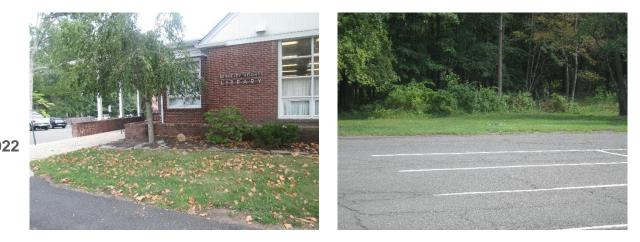
Parking spots east of the building can be replaced with porous asphalt to capture and infiltrate stormwater. A rain garden can be built adjacent to the parking lot to capture, treat, and infiltrate runoff. A preliminary soil assessment suggests that more soil testing would be required before determining the soil's suitability for green infrastructure.
