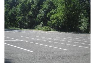
Multiple rows of parking spaces west of the school can be replaced with porous asphalt to capture and infiltrate stormwater. A preliminary soil assessment suggests that the soils have suitable drainage characteristics for green infrastructure.
