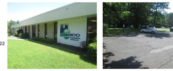
Parking spaces can be replaced with porous asphalt to capture and infiltrate stormwater runoff. A preliminary soil assessment suggests that more soil testing would be required before determining the soil's suitability for green infrastructure.
