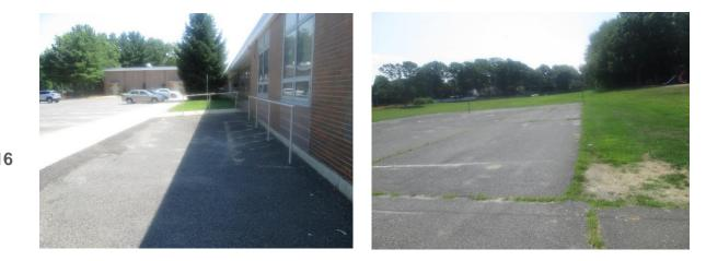
Parking spaces can be replaced with porous asphalt to infiltrate runoff. A rain garden can be installed adjacent to the building to capture, treat, and infiltrate roof runoff. A preliminary soil assessment suggests that the soils have suitable drainage characteristics for green infrastructure.
