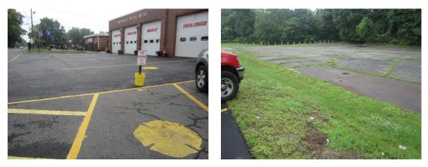
The turf grass area to the south of the parking garage appears feasible to construct a rain garden to receive runoff from a portion of the western parking lot. This green infrastructure practice will capture, treat, and infiltrate stormwater. A preliminary soil assessment suggests that the soils have suitable drainage characteristics for green infrastructure.
