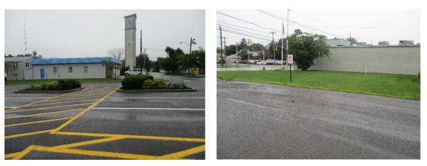
Runoff can be captured and treated by replacing the existing parking spaces with porous pavement. The site drains to an existing turf grass area to the east where a rain garden can be installed to filter and infiltrate stormwater runoff. A preliminary soil assessment suggests that the soils have suitable drainage characteristics for green infrastructure.
