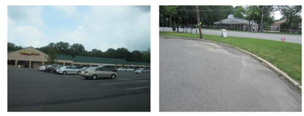
Two grassed islands at the parking lot entrance can be converted into rain gardens to help manage stormwater. These rain gardens will be aesthetically pleasing while capturing, treating, and infiltrating runoff. Parking spaces can be replaced with pervious pavement to capture and infiltrate stormwater. A preliminary soil assessment suggests that the soils have suitable drainage characteristics for green infrastructure.
