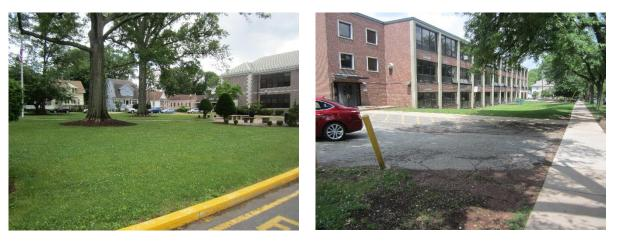
Several areas can be converted to porous pavement to infiltrate runoff. Downspouts on the southern end of the building can be disconnected to allow stormwater to infiltrate into an existing turf grass below. Another downspout can be disconnected a cistern to harvest rainwater, and a rain garden on the eastern side of the building can capture, treat, and infiltrate runoff. A preliminary soil assessment suggests that the soils have suitable drainage characteristics for green infrastructure.
