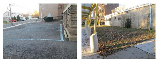
A bioretention system can be installed in the turf grass area near the entrance of the building capture, treat, and infiltrate rooftop runoff. The two downspouts in this area can be disconnected to direct stormwater from the building into the bioretention system. A preliminary soil assessment suggests that the soils have suitable drainage characteristics for green infrastructure.
