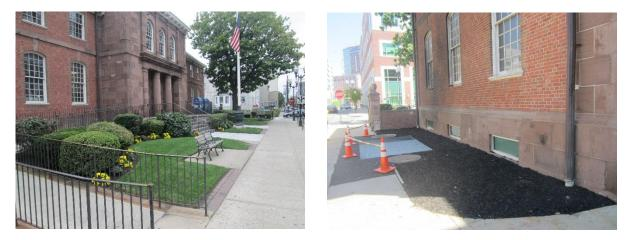
A bioretention system can be installed in front of the post office to capture, treat, and infiltrate rooftop runoff by redirecting the nearby downspout into it. A preliminary soil assessment suggests that more soil testing would be required before determining the soil's suitability for green infrastructure.
