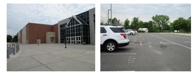
The high school is new with internal drainage. Parking spaces can be replaced with pervious pavement to capture and infiltrate stormwater. Rain gardens can also capture, treat, and infiltrate runoff. A preliminary soil assessment suggests that more soil testing would be required before determining the soil's suitability for green infrastructure.
