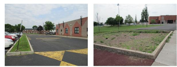
Parking spaces and the asphalt adjacent to the playground can be converted into pervious pavement to infiltrate stormwater. A preliminary soil assessment suggests that more soil testing would be required before determining the soil's suitability for green infrastructure.
