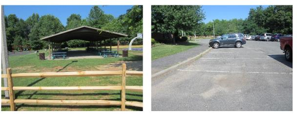
Stormwater is currently directed to an existing detention basin. Parking spots near the basketball courts can be replaced with porous asphalt to capture and infiltrate stormwater. A rain garden can be installed adjacent to the pavilion to capture, treat, and infiltrate roof runoff. A preliminary soil assessment suggests that the soils have suitable drainage characteristics for green infrastructure.
