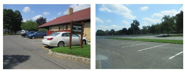
Parking spaces can be replaced with pervious pavement to capture and infiltrate stormwater. A rain garden can be installed to capture, treat, and infiltrate roof runoff. A preliminary soil assessment suggests that more soil testing would be required before determining the soil's suitability for green infrastructure.
