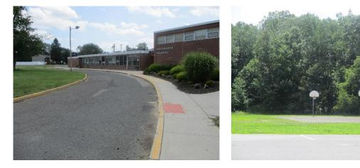
The existing basketball court and a row of parking spaces can be replaced with porous asphalt to capture and infiltrate stormwater. A preliminary soil assessment suggests that more soil testing would be required before determining the soil's suitability for green infrastructure.
