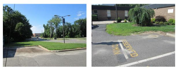
Stormwater is currently directed to an existing detention basin. Bioretention systems can be installed to capture, treat, and infiltrate parking lot runoff. Parking spaces can be replaced with pervious pavement to capture and infiltrate stormwater. A preliminary soil assessment suggests that the soils have suitable drainage characteristics for green infrastructure.
