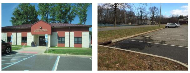
Multiple rows of parking spaces around the complex can be replaced with porous asphalt to capture and infiltrate stormwater. A rain gardens can be installed east of the library to capture, treat, and infiltrate roof runoff. A preliminary soil assessment suggests that more soil testing would be required before determining the soil's suitability for green infrastructure.
