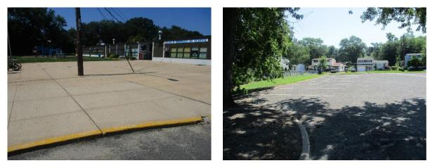
Parking spots northeast of the school can be replaced with porous asphalt to capture and infiltrate stormwater. A rain garden can be installed to capture, treat, and infiltrate rooftop runoff. A preliminary soil assessment suggests that the soils have suitable drainage characteristics for green infrastructure.
