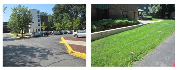
Parking spots north of the building can be replaced with porous asphalt to capture and infiltrate stormwater. A rain garden adjacent to the west side of the building can capture, treat, and infiltrate runoff. A preliminary soil assessment suggests that the soils have suitable drainage characteristics for green infrastructure.
