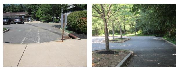
Parking spots west of the office suites can be replaced with porous asphalt to capture and infiltrate stormwater. A preliminary soil assessment suggests that the soils have suitable drainage characteristics for green infrastructure.
