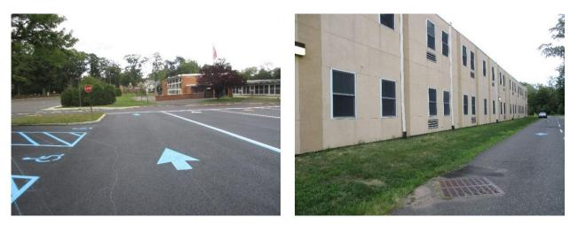
Parking spaces can be replaced using pervious pavement to allow stormwater to infiltrate. A rain garden can also be installed to capture, treat, and infiltrate roof runoff. A preliminary soil assessment suggests that more soil testing would be required before determining the soil's suitability for green infrastructure.
