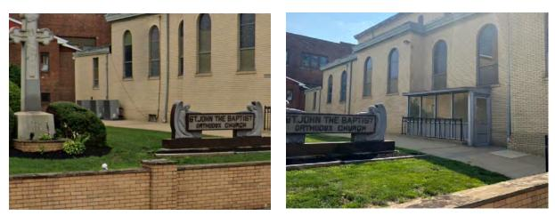
A rain garden can be installed in the central area between the buildings to capture, treat, and infiltrate stormwater runoff from the roof. A preliminary soil assessment suggests that more soil testing would be required before determining the soil's suitability for green infrastructure.
