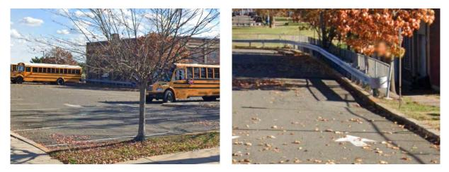
A section of the parking lot spaces can be converted to pervious pavement to intercept the stormwater flowing into the catch basin. A preliminary soil assessment suggests that more soil testing would be required before determining the soil's suitability for green infrastructure.
