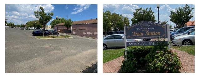
Parking spaces in the north and south portion of the parking lot can be converted to pervious pavement to help capture and infiltrate the stormwater runoff from the parking lot. A preliminary soil assessment suggests that more soil testing would be required before determining the soil's suitability for green infrastructure.
