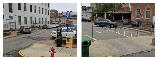
Western parking spaces in the parking lot can be converted to porous pavement to capture and infiltrate stormwater runoff from the parking lot. A preliminary soil assessment suggests that more soil testing would be required before determining the soil's suitability for green infrastructure.
