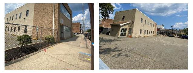
The existing planter bed can be converted to a rain garden to capture, treat, and infiltrate the stormwater from the existing downspout. A section of the parking lot spaces in the southeastern corner can be converted to pervious pavement to capture and infiltrate the stormwater runoff from the parking lot. A preliminary soil assessment suggests that more soil testing would be required before determining the soil's suitability for green infrastructure.
