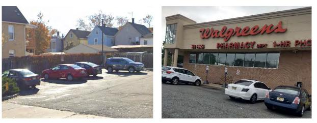
Parking lot spaces to the east and west of the building can be converted to pervious pavement to capture and infiltrate the stormwater runoff from the parking lot. A preliminary soil assessment suggests that more soil testing would be required before determining the soil's suitability for green infrastructure.
