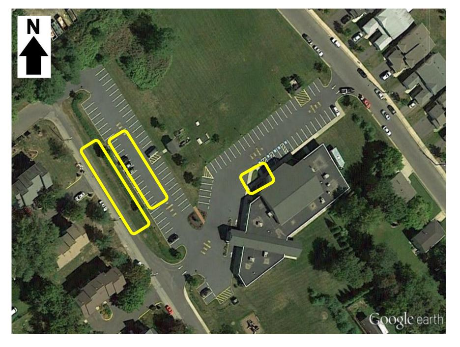
**BIORETENTION SYSTEMS:** A bioretention system can be installed near the front entrance of the church to intercept runoff from the rooftop. Another bioretention system can be installed along Spruce Street to mitigate erosion and sediment buildup. The gardens can also provide habitat for birds, butterflies, and pollinators.
