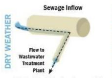
Water is held in the pipes and flows to treatment plant.
