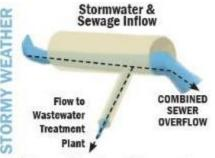
The combination of stormwater and sewage exceeds capacity and overflows into local waterways
