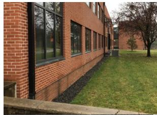
A rain garden can be installed in the turfgrass area near the southeast entrance of Grant Hall to capture, treat, and infiltrate stormwater runoff from the roof. Similar rain gardens could be installed at other locations throughout the campus. A preliminary soil assessment suggests that more soil testing would be required before determining the soil's suitability for green infrastructure.
