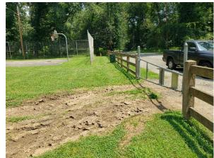
Rain gardens can be installed in the turfgrass area near the entrance of the park and the basketball court to capture, treat, and infiltrate stormwater runoff from the parking area and the basketball court, respectively. A preliminary soil assessment suggests that more soil testing would be required before determining the soil's suitability for green infrastructure.
