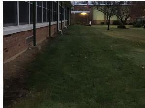
Rain gardens can be installed in the turfgrass areas at several locations around the building by redirecting downspouts into them to capture, treat, and infiltrate stormwater runoff from the roof. A preliminary soil assessment suggests that more soil testing would be required before determining the soil's suitability for green infrastructure.
