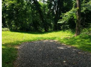
A rain garden can be installed in the turfgrass area between the basketball court and gravel driveway to capture, treat, and infiltrate stormwater runoff from the basketball court. A preliminary soil assessment suggests that more soil testing would be required before determining the soil's suitability for green infrastructure.
