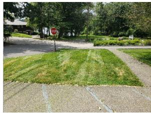
Rain gardens can be installed in the turfgrass areas in the island west of the building's front and in the southeast corner of the building to capture, treat, and infiltrate stormwater runoff from the parking lot and roof, respectively. A preliminary soil assessment suggests that more soil testing would be required before determining the soil's suitability for green infrastructure.
