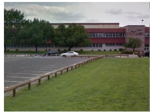
Rain gardens can be installed in the turfgrass areas in the islands to the west of the building to capture, treat, and infiltrate stormwater runoff from the roadway and gravel parking lot. A preliminary soil assessment suggests that more soil testing would be required before determining the soil's suitability for green infrastructure.
