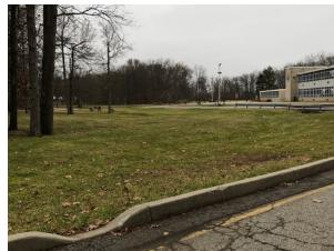
A rain garden can be installed in the turfgrass area near the driveway off Lenox Road to capture, treat, and infiltrate stormwater runoff from the pavement. A portion of the parking spaces in the center of the parking lot can be retrofitted with pervious pavement to capture runoff from the rest of the parking lot. A preliminary soil assessment suggests that more soil testing would be required before determining the soil's suitability for green infrastructure.
