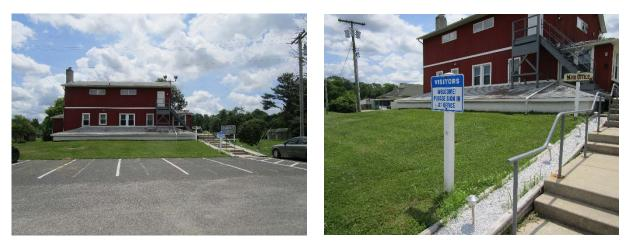
Two rain gardens can be installed in the turfgrass area on each side of the building to capture, treat, and infiltrate runoff from the roof of the building while also providing aesthetic value. A preliminary soil assessment suggests that more soil testing would be required before determining the soil's suitability for green infrastructure.
