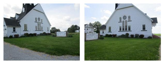
Rain gardens can be installed in the turfgrass area at the front of the church and behind the church. The gardens would capture, treat, and infiltrate runoff from the roof of the building and the parking area. A preliminary soil assessment suggests that the soils have suitable drainage characteristics for green infrastructure.
