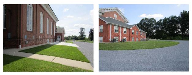
Three rain gardens can be installed in the grassed area adjacent to the church building to capture runoff from the roof of the building. Pervious pavement can also be installed in the parking spaces at the back of the building to capture and treat runoff from the surrounding pavement. A preliminary soil assessment suggests that the soils have suitable drainage characteristics for green infrastructure.
