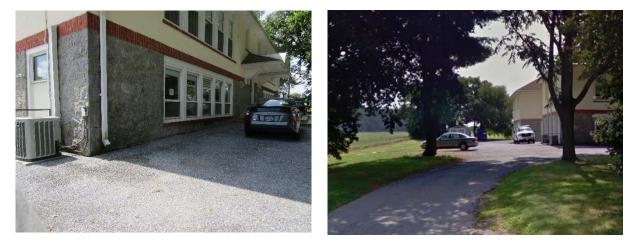
Pervious pavement can be installed in the parking spaces northeast of the school to capture, treat, and infiltrate runoff from the roof of the building and parking lot instead of flowing into the street and into a nearby catch basin. A preliminary soil assessment suggests that the soils have suitable drainage characteristics for green infrastructure.
