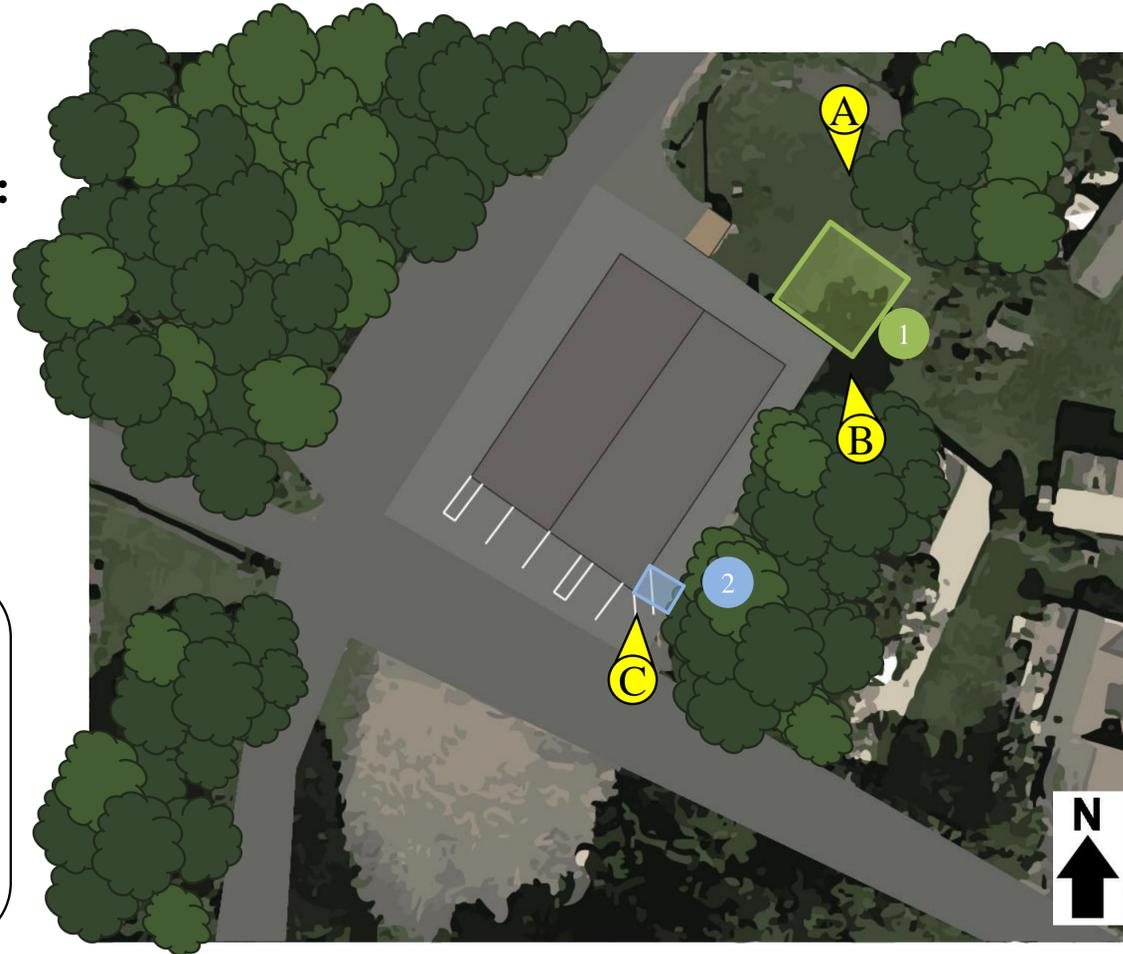
**1 BIORETENTION SYSTEM:** A rain garden can be used on this property to reduce sediment and nutrient loading to the local waterway and increase groundwater recharge. A rain garden can be implemented at the rear of the building to capture runoff from the rooftop.
