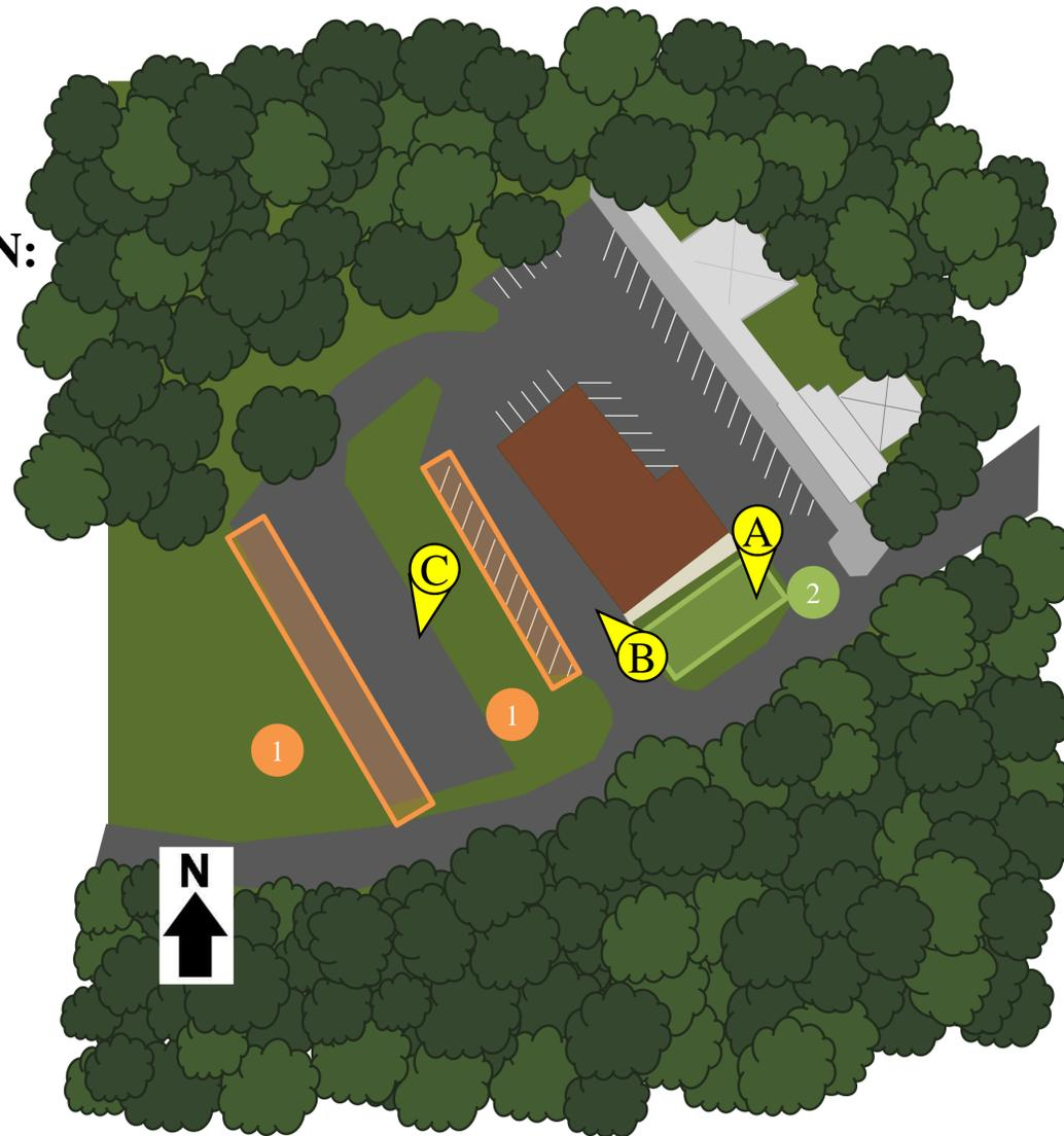
**1 POROUS PAVEMENT:** Porous pavement promotes groundwater recharge and filters stormwater. The parking spots along the southwest end of the building can be redone to capture rooftop and driveway runoff, and the additional parking area can receive a strip of porous pavement to capture additional runoff.
