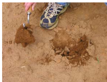
Insert the trowel or spade to a depth of 3, 6, 9, or 12 inches, remove some soil and set it aside.
