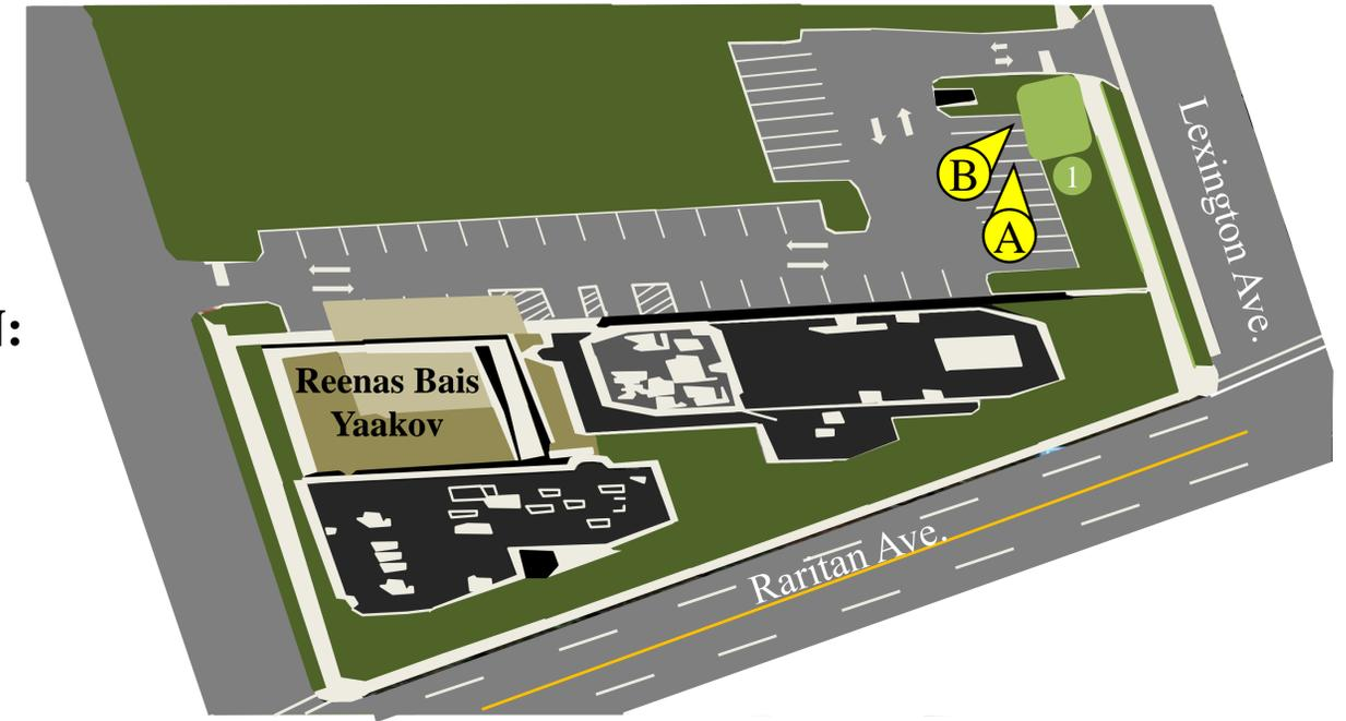
**1 BIORETENTION SYSTEMS:** A bioretention system could be installed on the turf grass area parallel to Lexington Avenue. This would capture, treat, and infiltrate stormwater runoff from the parking lot.
