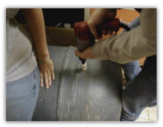
Drill where barrel is flat, not near a seam.
