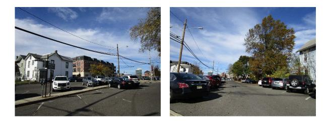
Parking spaces can be replaced with porous asphalt to capture and infiltrate stormwater. A preliminary soil assessment suggests that the soils have suitable drainage characteristics for green infrastructure.
