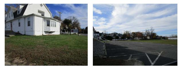
Parking spots to the north of the building can be replaced with porous asphalt to capture and infiltrate stormwater. Installing a rain garden adjacent to the building can capture, treat, and infiltrate roof runoff. A preliminary soil assessment suggests that the soils have suitable drainage characteristics for green infrastructure.
