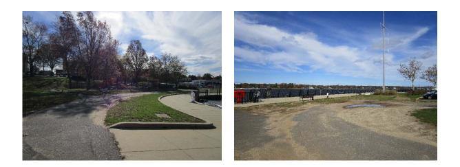
Parking spots to the north end can be replaced with porous asphalt to capture and infiltrate stormwater. Installing rain gardens in the eroded areas around the park can capture, treat, and infiltrate runoff from the parking lot and walkways. A preliminary soil assessment suggests that the soils have suitable drainage characteristics for green infrastructure.
