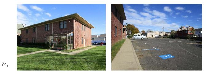
Parking spots to the east of the building can be replaced with porous asphalt to capture and infiltrate stormwater from downspouts already discharging to them. Installing rain gardens adjacent to the building can capture, treat, and infiltrate roof runoff. A preliminary soil assessment suggests that the soils have suitable drainage characteristics for green infrastructure.
