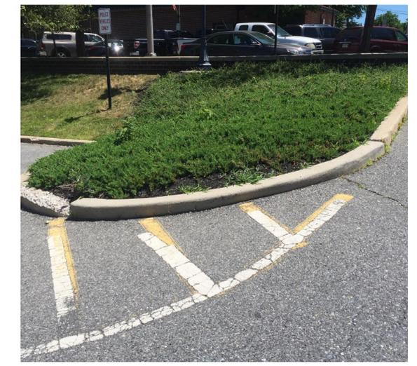
**1 BIORETENTION SYSTEMS:** Rain gardens can be used to reduce sediment and nutrient loading to the local waterway and increase groundwater recharge. This site has multiple areas where downspouts can be disconnected and rain gardens installed in the north parking lot area. Curb cuts can be made to allow stormwater to enter the bioretention systems from the street and parking lot.
